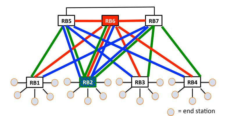
RBridges support multiple distribution trees. The encapsulating RBridge chooses which to use. RB2 can split multi-destination traffic over three trees.
